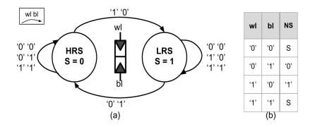
Next state NS is Boolean majority of the three inputs (M<sub>3</sub>) with the bitline input inverted.
