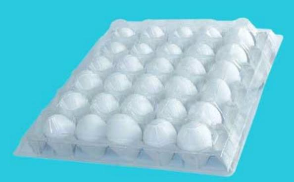
Vacuum forming, is a simplified version of thermoforming, whereby a sheet of plastic is heated to a forming temperature, stretched onto or into a single-surface mould, and held against the mould by applying vacuum between the
